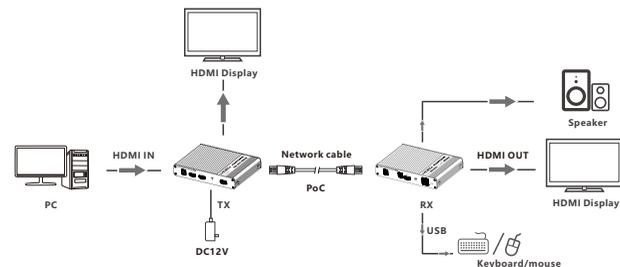
Follow the standard of IEEE-568B, It is recommended to select a network cable with less loss and crosstalk.
