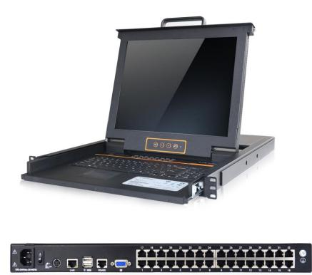
Featuring an integrated LCD monitor, keyboard, and touchpad in a 1U rack-mountable housing, the HT17xx LCD KVM over IP Switch is a control unit that allows secure access to 8/16/24/32 computers from a single KVM console.
