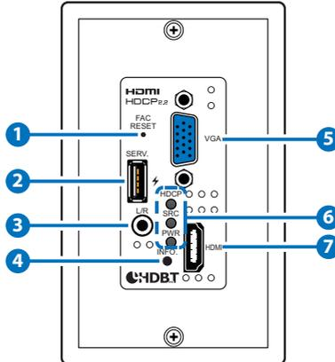
**1 FAC RESET Button:** Press and hold for 5 seconds to reset the unit to its factory defaults.
