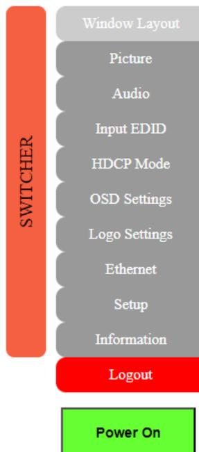
Clicking the red "Logout" tab will automatically log the currently connected user out of the WebGUI and return to login page. Clicking on the "Power" button will toggle the unit's current power state between on (green) and stand-by (red).
