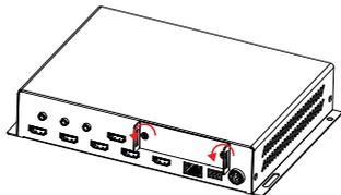
(2) Completely unscrew both screws.
