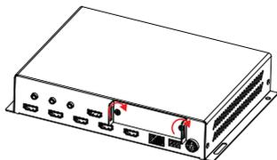
(4) Cover the module slot with a dummy faceplate and tighten both screws.
