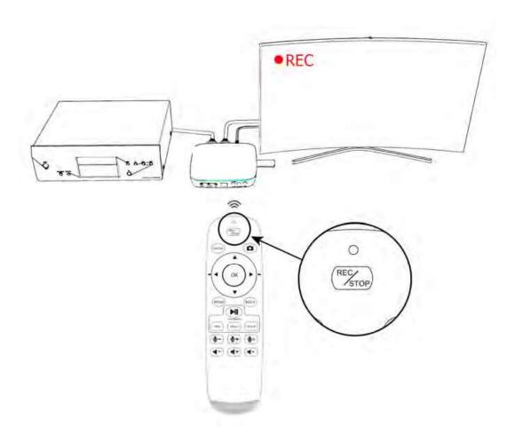
4. During recording process, you can adjust the volume of HDMI IN at any time. If you got Mic connected, you also can adjust the volume of Mic during recording by pressing the volume up/down button on the Remote.
