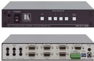
The VP-411DS is a high-performance switcher for computer graphics video signals, with resolutions up to and exceeding UXGA, and unbalanced stereo audio signals. When configured as a standby switcher, the switching priority can be set for each of the four inputs
