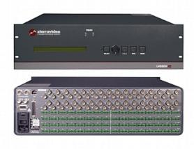
The Lassen HD XL Series offers flexibility and adaptability to any application where saving space and costs are important. 3232HDS-XL is a 32x32 HD-SDI (1.5G) & analog balanced stereo audio matrix switcher, available in a compact 3RU frame. 3232HDS-XL also supports breakaway stereo audio switching whereby the digital video, audio left and audio right can all be routed independently. It offers control via the front panel or remotely via RS-232 or Ethernet
