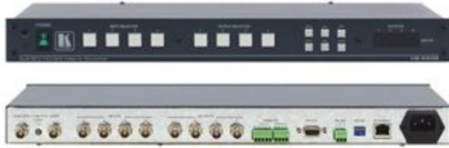
The VS-44HD is a high-performance 4x4 matrix switcher for HD-SD signals, as well as a dual link 2x2 matrix switcher. Switching is implemented during the vertical interval period according to the SMPTE RP-168 standard, when using synchronized digital video sources
