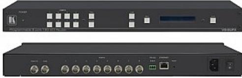
VS-8UFX is an 8-port matrix switcher for SDI signals for up to 12G SDI. Each SDI port can be defined as either an input or output, enabling flexible configurations such as a 1x7 distribution amplifier, 7x1 switcher, 4x4 matrix switcher or any other possible input-output combination. VS-8UFX is easy to operate and control through the network using the intuitive web pages and through RS-232 using a serial controller
