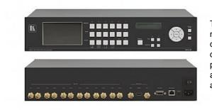
The MV-6 is a versatile, high-performance multiviewer for 3G HD-SDI video signals. The device can display up to six inputs in any combination and output the image in SDI, HDMI and CV formats. Both pre-programmed and customizable screen divisions are supported. The MV-6-MD is certified for medical applications
