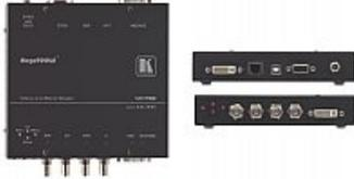
The VP-792 is a high-performance scaler for HDMI, DVI, analog VGA and component signals. It up- or down-scales the incoming signal, processes the image with HQV, flexible warping, geometry correction and edge blending and outputs the signal to a DVI/HDMI connector
