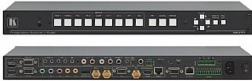
The VP-771 is a high-quality presentation switcher and scaler for a variety of signals. It accepts one of nine inputs: component video, DisplayPort (DP), 3G HD-SDI, two computer graphics, two composite video and two HDMI signals. It scales the video, embeds the audio, and outputs the signal to one HDMI, one computer graphics, one 3G HD-SDI and one DGKat TP, together with digital audio, unbalanced stereo and a 2x10-watt amplified balanced stereo speaker output
