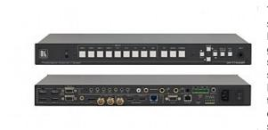
The VP-774AMP is a high-performance presentation switcher and scaler. It accepts one of nine inputs: one DisplayPort (DP), one composite video, two computer graphics, one 3G HD-SDI and four HDMI signals. It scales the video, embeds the audio, and simultaneously outputs the signal to two identical HDMI, one HDBaseT and one 3G HD-SDI output, together with S/PDIF and balanced stereo audio outputs. The unit also includes an audio amplifier and speaker outputs
