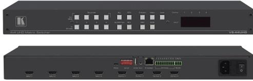
VS-44UHD is a high-quality 4x4 matrix switcher for 4K@60Hz (4:2:0) HDMI signals and embedded audio. It reclocks and equalizes the signals and can route any one of four HDMI, HDCP-compliant sources (selectable) to any or all outputs simultaneously. VS-44UHD offers a flexible audio scheme where any HDMI digital audio input can be routed to any HDMI digital audio output in addition to ARC support on all ports to produce an equivalent 8x8 audio matrix
