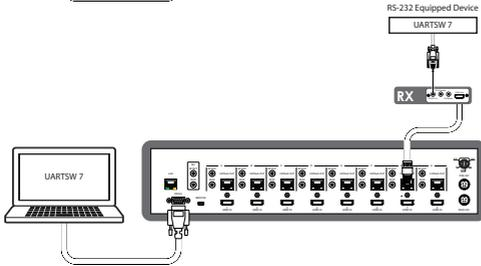
**Note:** This command allows RS-232 to control the RS-232 device connected to output G's Receiver.
