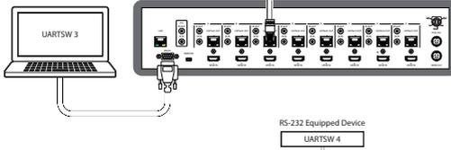
**Note:** This command allows RS-232 to control the RS-232 device connected to output C's Receiver.
