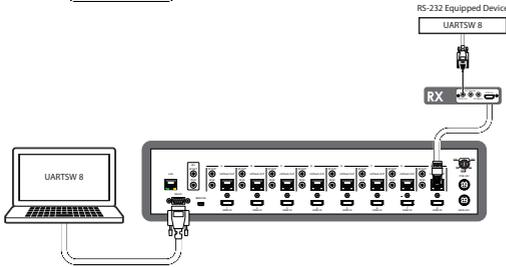
**Note:** This command allows RS-232 to control the RS-232 device connected to output H's Receiver.
