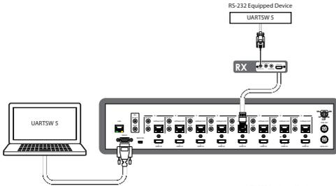
**Note:** This command allows RS-232 to control the RS-232 device connected to output E's Receiver.
