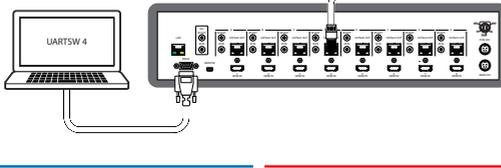
**Note:** This command allows RS-232 to control the RS-232 device connected to output D's Receiver.
