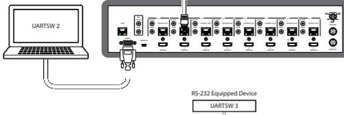
**Note:** This command allows RS-232 to control the RS-232 device connected to output B's Receiver.
