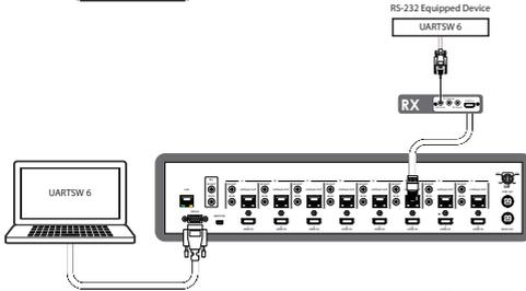
**Note:** This command allows RS-232 to control the RS-232 device connected to output F's Receiver.
