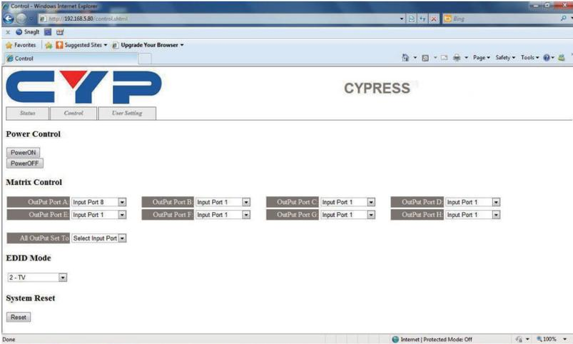
Clicking on the 'User Setting' tab allows you to reset the IP configuration. The system will ask for a reboot of the device every time any of the settings are changed. The IP address needed to access the Web GUI control will also need to be changed accordingly on the web address entry bar.
