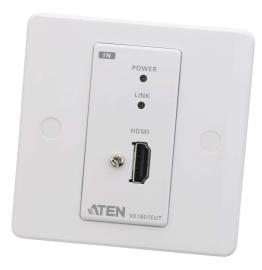
ATEN VE1801EUT is a transmitter designed to reliably send 4K signals up to 40 m over a single Cat 5e/6/6a or ATEN 2L-2910 Cat 6 cable. With EU Wall Plate design, the VE1801EUT can be conveniently mounted in a one-gang junction box. For HDMI signal transmission, it supports 3D, Deep Color, and embedded HD lossless audio formats.
