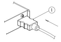
2. Loosen the port screw slightly.
