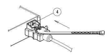
5. Tightly wrap the tail of the LockPro around the narrowest part of the HDMI cable. Securely connect the LockPro tail to the LockPro head via the buckle mechanism. Make sure it clips into place and cannot come loose.
