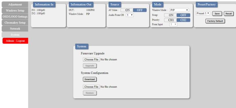
1) **System:** This section contains all controls relating to firmware upgrades and system configuration export.
