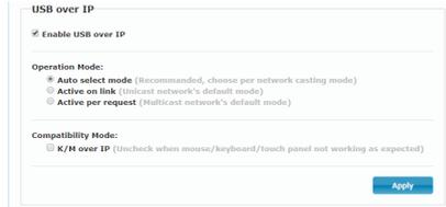
The screenshot shows a configuration panel titled "USB over IP". It contains three sections: "Enable USB over IP" with a checked checkbox, "Operation Mode" with three radio button options (Auto select mode, Active on link, Active per request), and "Compatibility Mode" with one checked checkbox (K/M over IP). An "Apply" button is located at the bottom right.
