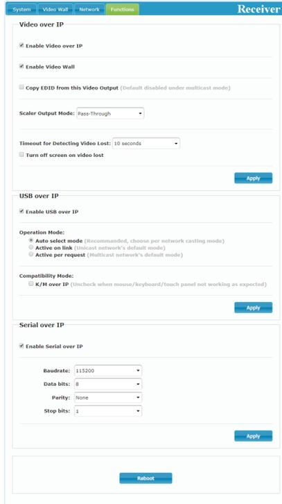
The screenshot shows the 'Receiver' web interface with the 'Functions' tab selected. The interface is divided into three main sections: 'Video over IP', 'USB over IP', and 'Serial over IP'. Each section contains various configuration options and an 'Apply' button. At the bottom of the page is a 'Reboot' button.
