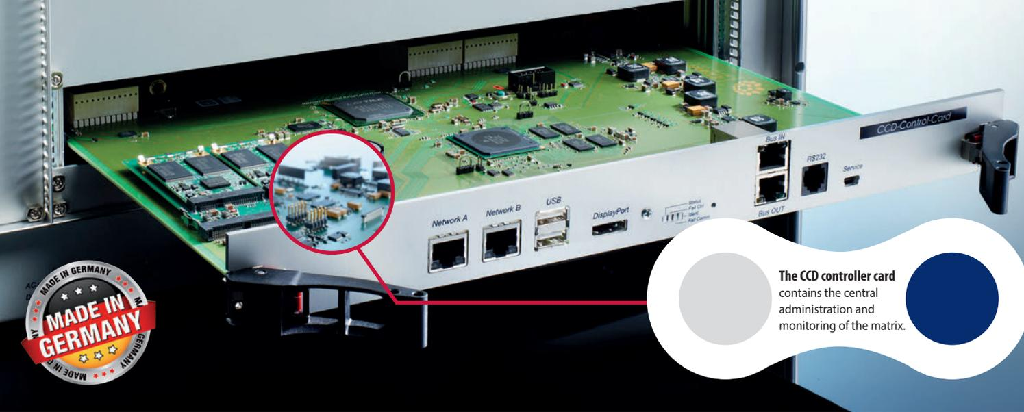
The CCD controller card contains the central administration and monitoring of the matrix.
