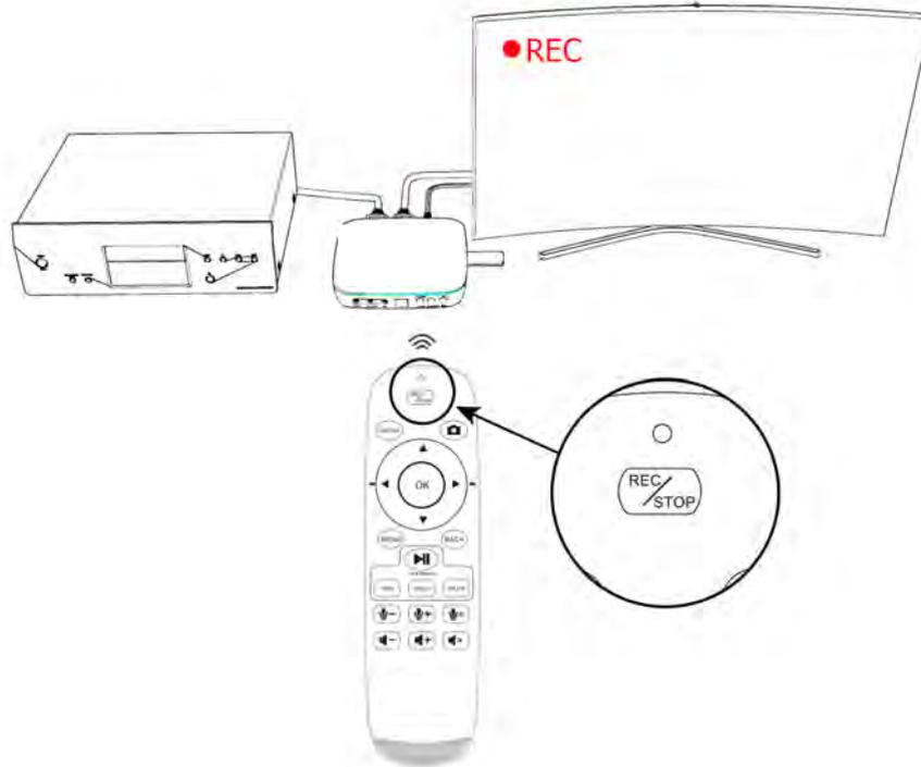
4. During recording process, you can adjust the volume of HDMI IN at any time. If you got Mic connected, you also can adjust the volume of Mic during recording by pressing the volume up/down button on the Remote.
