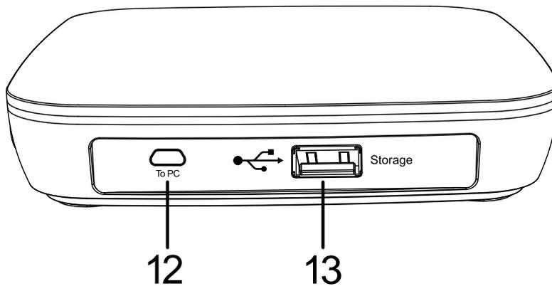
12. TO PC Connect the Micro-USB to USB cable between PC and UHD for recording video to PC
