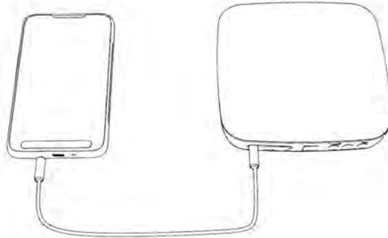
After connected audio device to “Line in” , it will directly mix audio to HDMI embedded audio. It also can be monitored from “Line out” and output devices.
