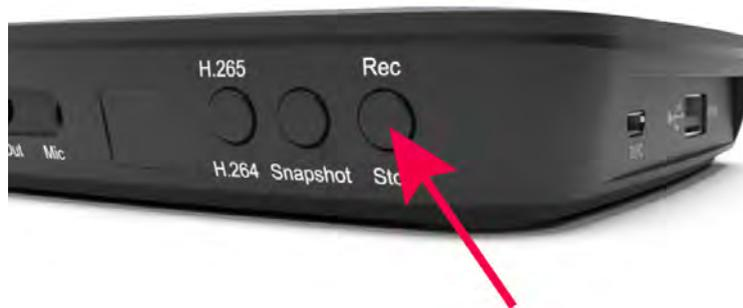
4. Press the Rec/Stop button again on UHD Pro, then the LED will blink blue/green alternately, which indicates the recorded video is being saved.
