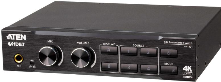
The ATEN VP1421 is a multi-in-one [presentation switch](#) that integrates a [video matrix](#) switch, 4K scaler, HDBaseT extender, audio DSP, and [analog](#)-to-digital converter functions into one compact device that easily mounts under a table or in a rack. With four [analog](#)/digital inputs to one HDBaseT and one HDMI [True 4K](#) outputs, it is designed to boost the efficiency and impact of professional [presentations](#).
