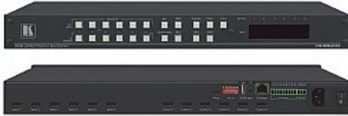
VS-66UHD is a high-quality 6x6 matrix switcher for 4K@60Hz (4:2:0) HDMI signals and embedded audio. It reclocks and equalizes the signals and can route any one of six HDMI, HDCP-compliant sources (selectable) to any or all outputs simultaneously. VS-66UHD offers a flexible audio scheme where any HDMI digital audio input can be routed to any HDMI digital audio output in addition to ARC support to produce an equivalent 12x9 audio matrix
