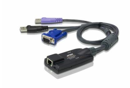
The KA7177 KVM Adapter Cable connects the KVM switch to the video and USB ports of the target computer. The KA7177 also provides a USB plug to connect the target computer for Smart Card/CAC support. With its small form factor and light weight design, it represents the next generation of KVM Adapter Cables – offering superior signal compensation and delay skew techniques for greatly enhanced video quality.
