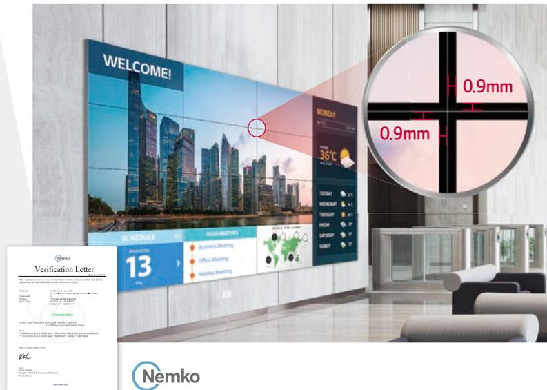
\* The 0.9mm even panel bezel and 1.8mm BtB size (borderless type, no metal bezel) have been verified by Nemko, a global institution that tests and certifies electrical equipment.
