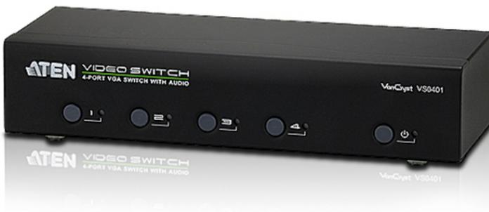
The VS0401 4-Port VGA Switch with Audio allows you to connect four audio/video source computers to a single monitor or projector with full audio and quickly switch between the devices for use.
